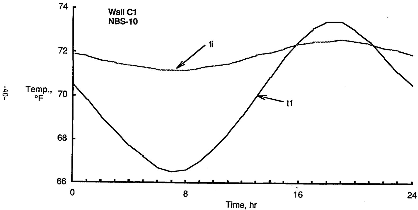
Fig. 22 Measured Indoor Air and Surface Temperatures for NBS-10 Test Cycle Applied to Wall C1
