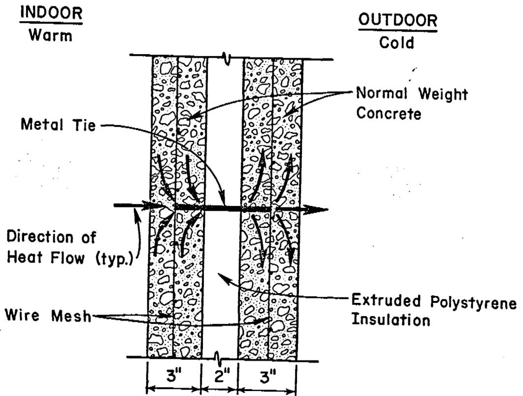
Fig. 2 Thermal Bridge Due to Metal Tie Penetrating Insulation
