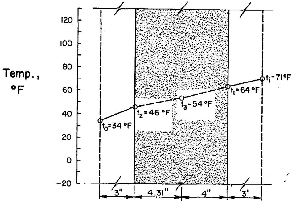
(a) Mean Wall Temperature =  $55^\circ\text{F}$
