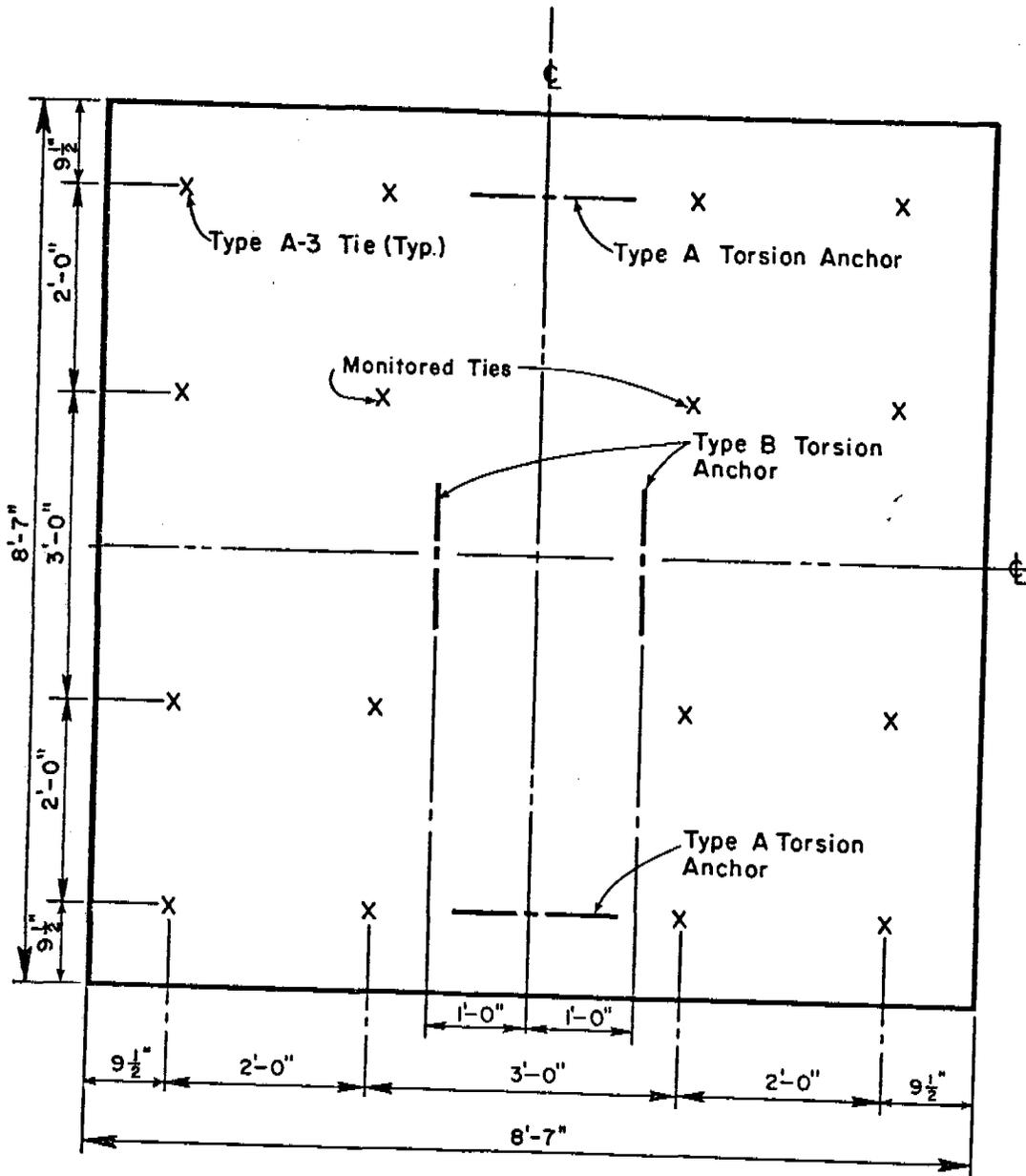
Fig. 3 Location of Stainless Steel Torsion Anchors and Ties in Wall P2
