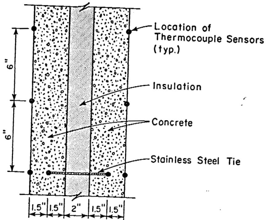
Fig. 10 Locations of Thermocouples in Vicinity of Stainless Steel Tie
