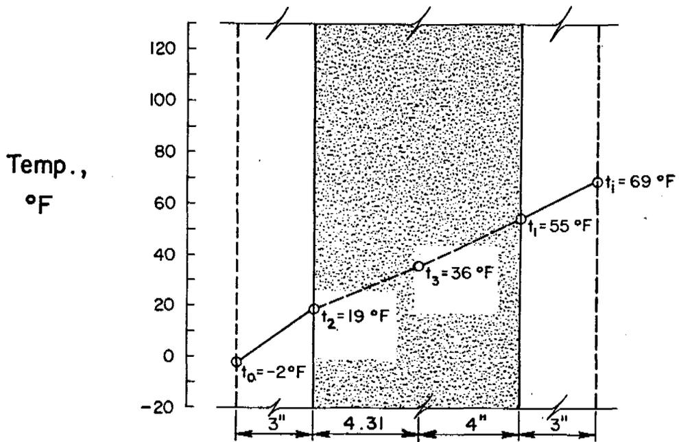
(b) Mean Wall Temperature =  $37^\circ\text{F}$
