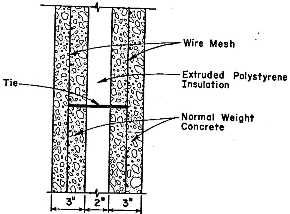
Fig. 1 Cross Section of Insulated Sandwich Panel Walls
