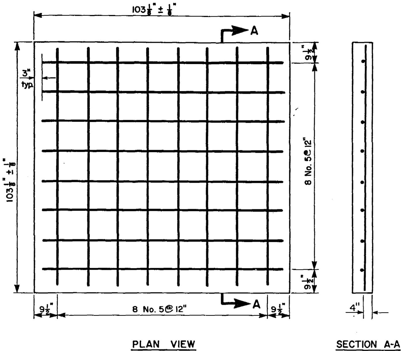
Fig. 7 Reinforcement Details for Normal-Weight Concrete Wall C1
