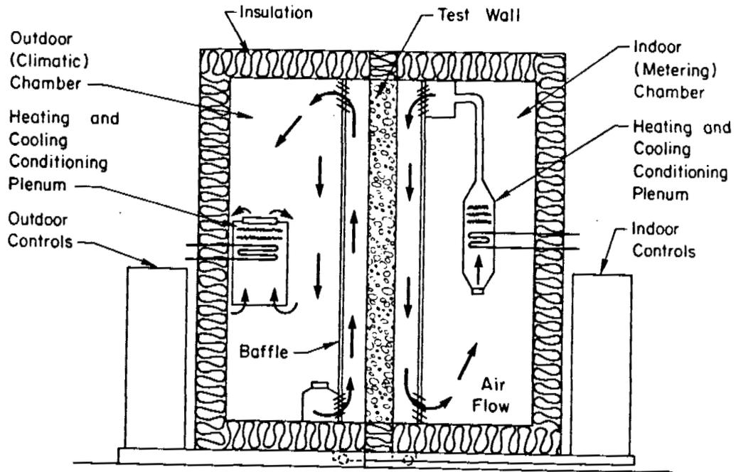
Fig. 12 Schematic of Calibrated Hot Box
