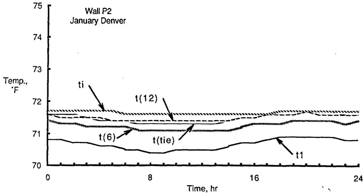
Fig. 21 Measured Indoor Air and Surface Temperatures for January Denver Test Cycle Applied to Wall P2
