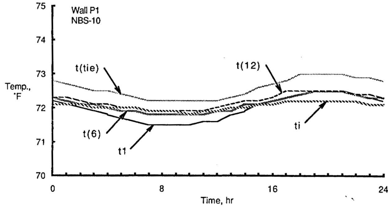
Fig. 19 Measured Indoor Air and Surface Temperatures for NBS-10 Test Cycle Applied to Wall P1
