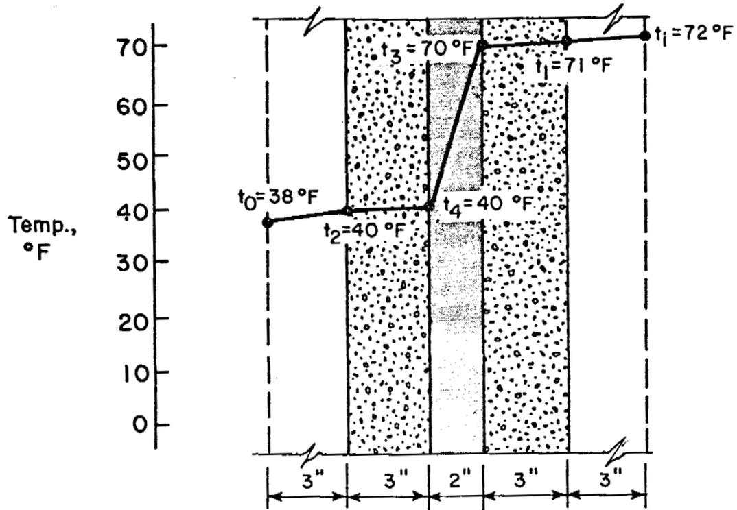
(a) Mean Wall Temperature =  $56^\circ\text{F}$
