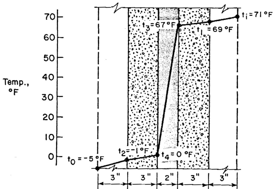
(b) Mean Wall Temperature =  $34^\circ\text{F}$
