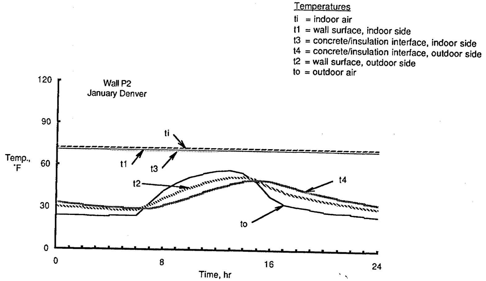
Fig. A1 Measured Temperatures for January Denver Test Cycle Applied to Wall P2
