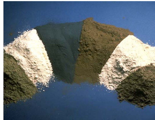
Fig.4 Supplementary cementitious materials. From left to right, fly ash (Class C), metakaolin (calcined clay), silica fume, fly ash (Class F), slag cement, and calcined shale. Photo courtesy of the Portland Cement Association.
