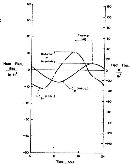
Fig. 3. Definition of Thermal Lag and Reduction in Amplitude
