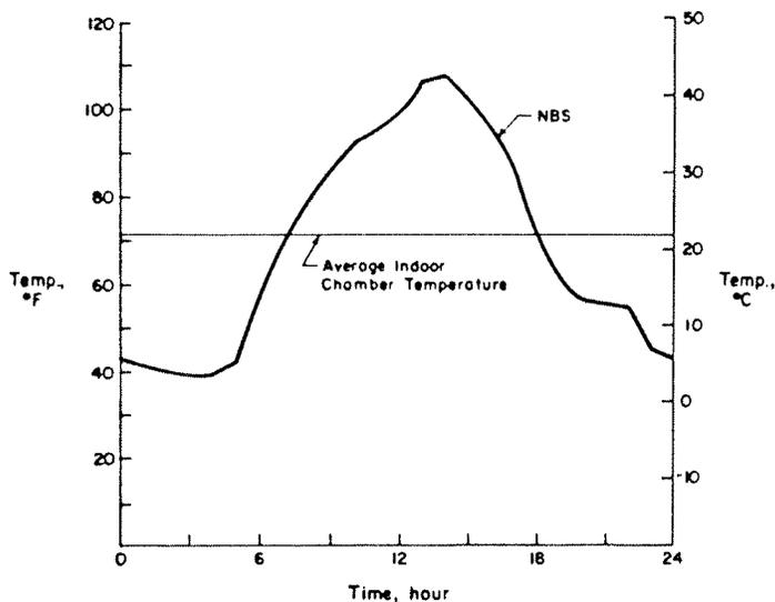
Fig. 2. Outdoor Chamber Air Temperature for NBS Dynamic Test Cycle
