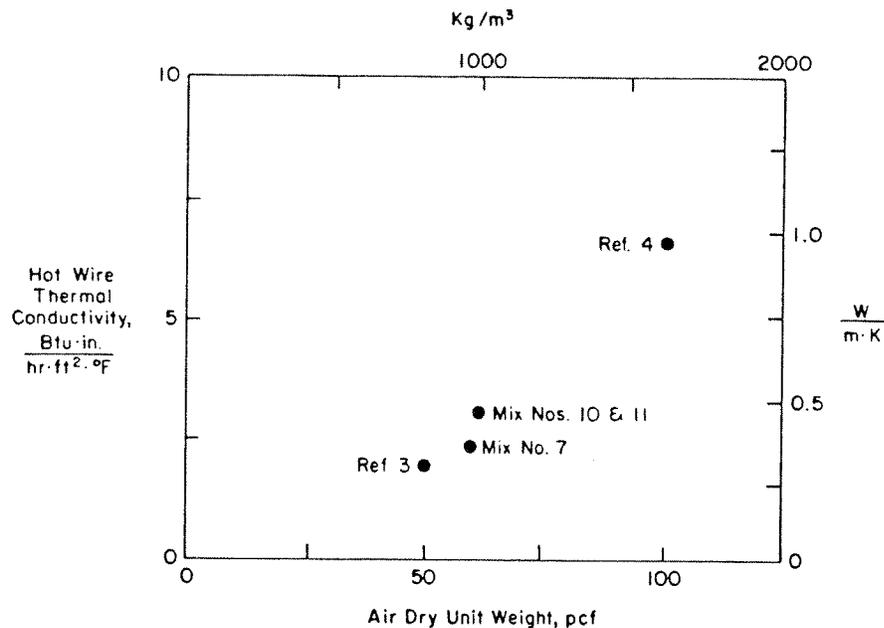
Fig. 1. Results from Hot Wire Thermal Conductivity Tests on Air Dry Specimens
