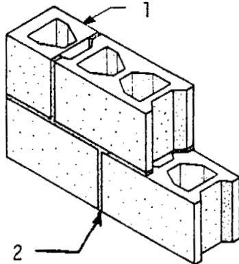
1. 8x8x16-in. (203x203x406-mm) Medium Weight Hollow Core Concrete Block - 2 cores per block
