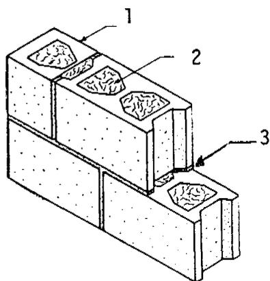
1. 8x8x16-in. (203x203x406-mm) Medium Weight Hollow Core Concrete Block - 2 cores per block
