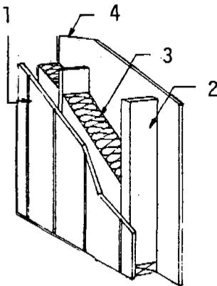
1. 7/16-in. (11-mm) Medium Density Hardboard Siding with vertical grooves spaced 8 in. (203 mm) on centers
