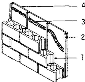
1. 8x8x16-in. (203x203x406-mm) Lightweight Hollow Core Concrete Block - 2 cores per block
