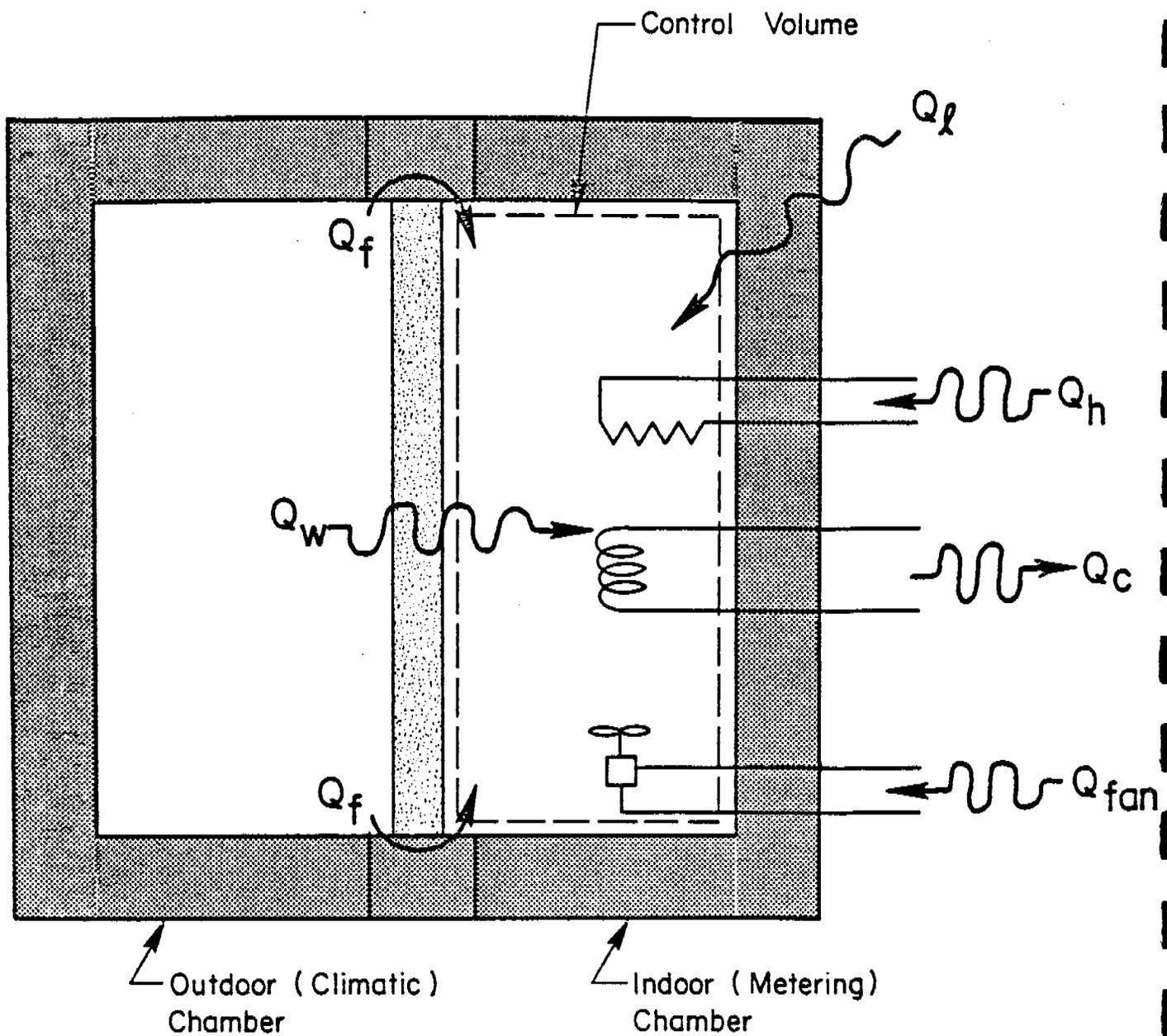
Fig. 3 Indoor (Metering) Chamber Energy Balance
