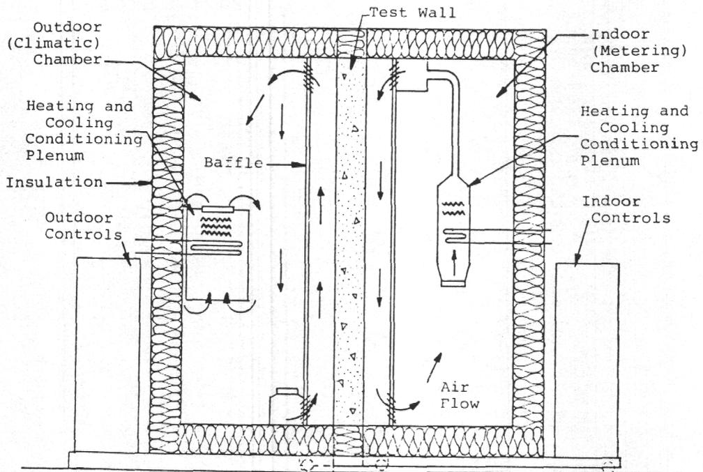
Fig. 2 Schematic of Calibrated Hot Box
