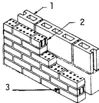
1. 4x8x16-in. (102x203x406-mm) Medium Weight Hollow Core Concrete Block - 3 cores per block
