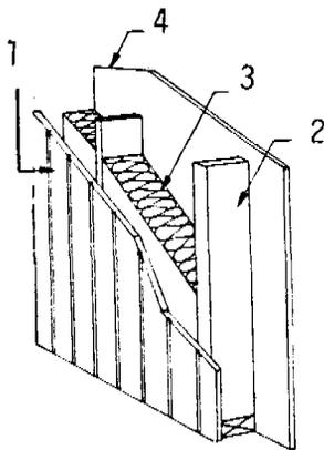
1. 5/8-in. (16-mm) Plywood Cedar Siding with rough sawn surface and vertical grooves at 8-in. (203-mm) on centers
