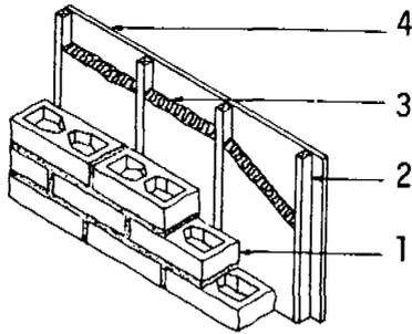
1. 8x4x16-in. (203x102x406-mm) Normal Weight Hollow Core Concrete Slump Block - 2 cores per block
