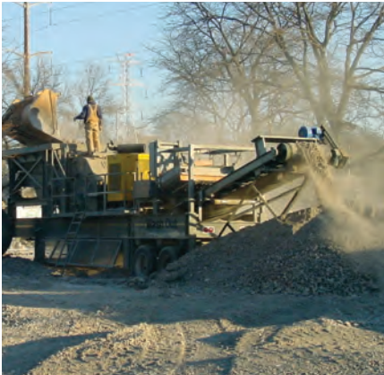
Left: Crushing concrete for reuse (photo: CTLGroup). Right: On-site collection of construction materials for recycling (photo: GSA).
