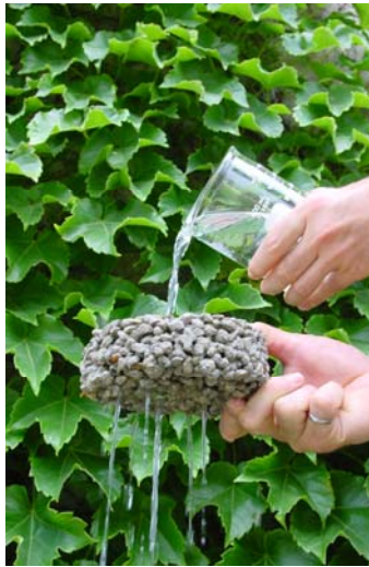
Figure 1. Water flows through pervious concrete.
