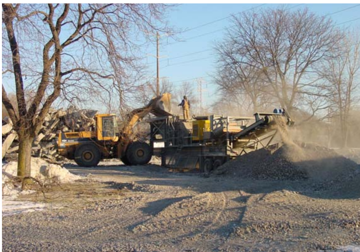
Figure 4. Recycled concrete can be reused as aggregate for new concrete, as sub-base material, and as erosion control.
