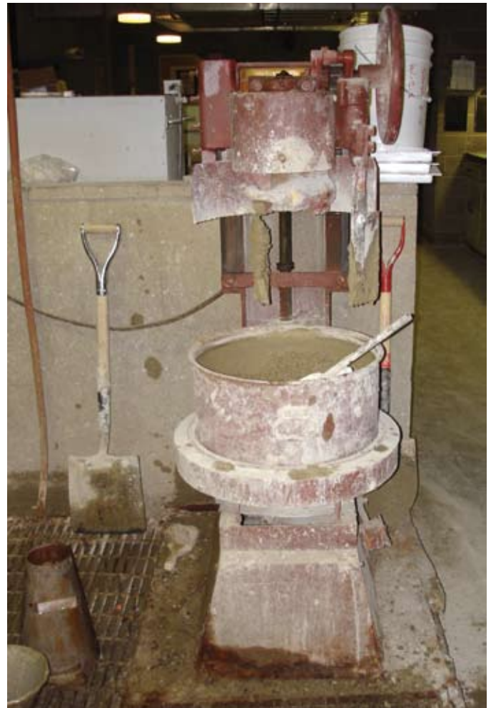
Fig. 4: The 0.5 ft 3 (0.014 m 3 ) pan mixer used to mix concrete for the specimens
