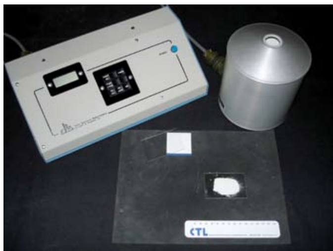
Fig. 3: Solar spectrum reflectometer used to measure solar reflectance of the constituent materials and concrete surfaces in this study. The measurement head is the cylindrical piece in the upper right corner
