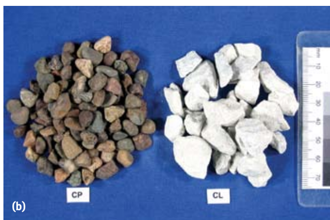
Fig. 2: Aggregates used in the current study: (a) fine aggregates; and (b) coarse aggregates. Numbers on each fine aggregate sample indicate the solar reflectance of the material
