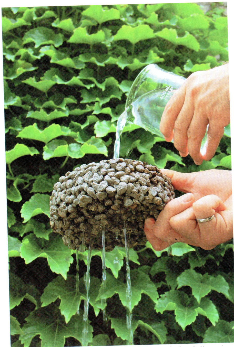
Figure 1. Water flows freely through pervious pavement because it contains an abundance of voids.
