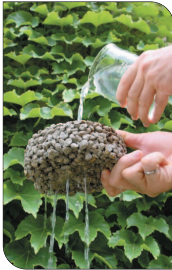
Sustainable Sites Credit 6.1. Water flows freely through a section of pervious pavement.
