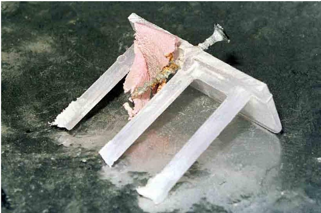
**Figure 29. Close-up of a corroded drywall screw showing corrosion only occurs on the portion of the screw embedded in the polystyrene.**
