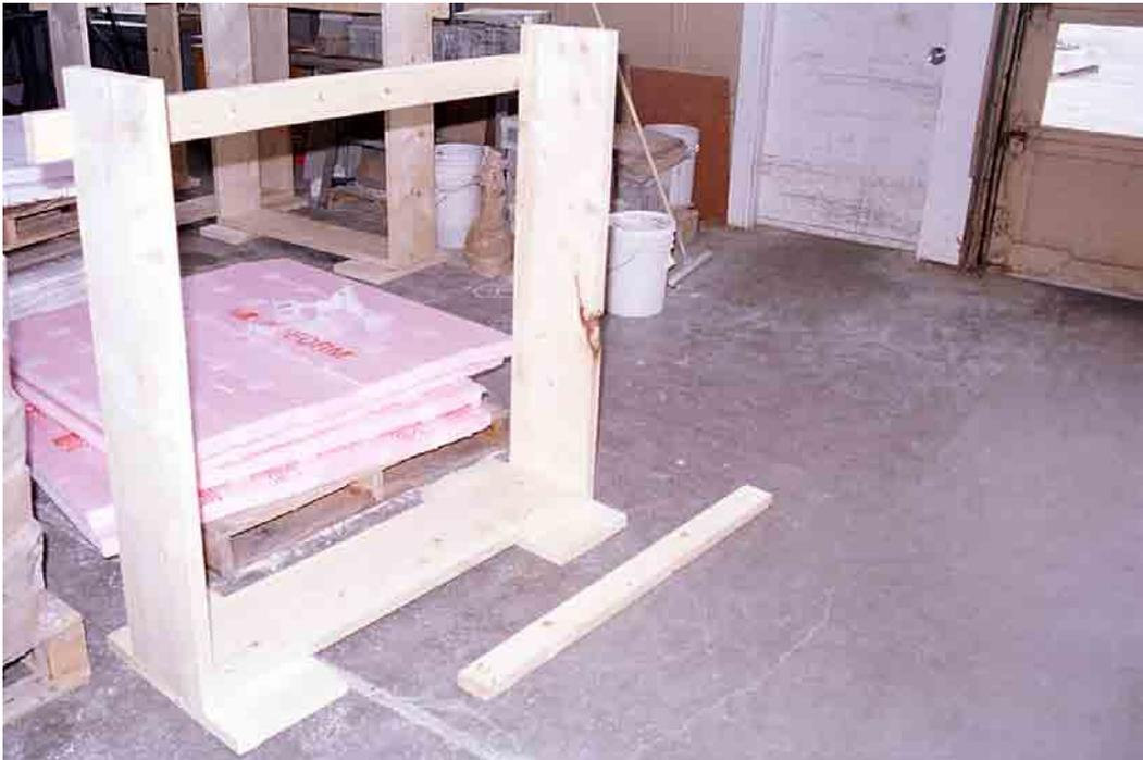
**Figure 1. Wood form for ICF wall section.**
