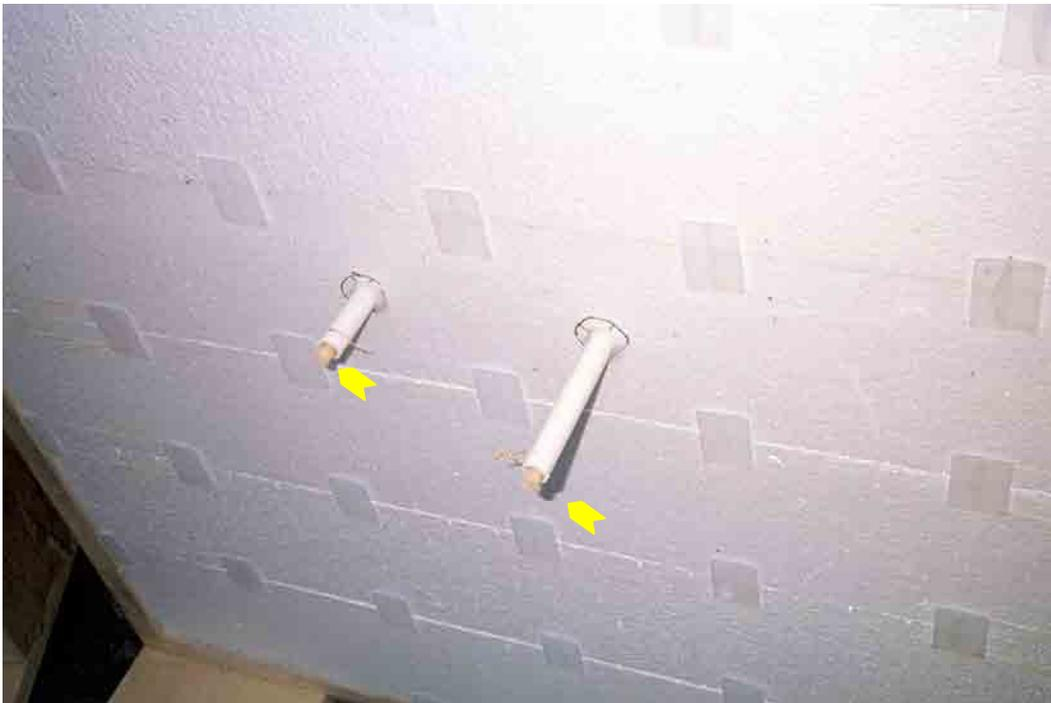
**Figure 8. Temporary plugs installed in relative humidity measurement ports.**
