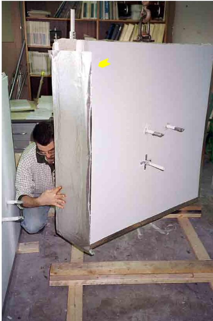
**Figure 24. Application of edge sealing material.**
