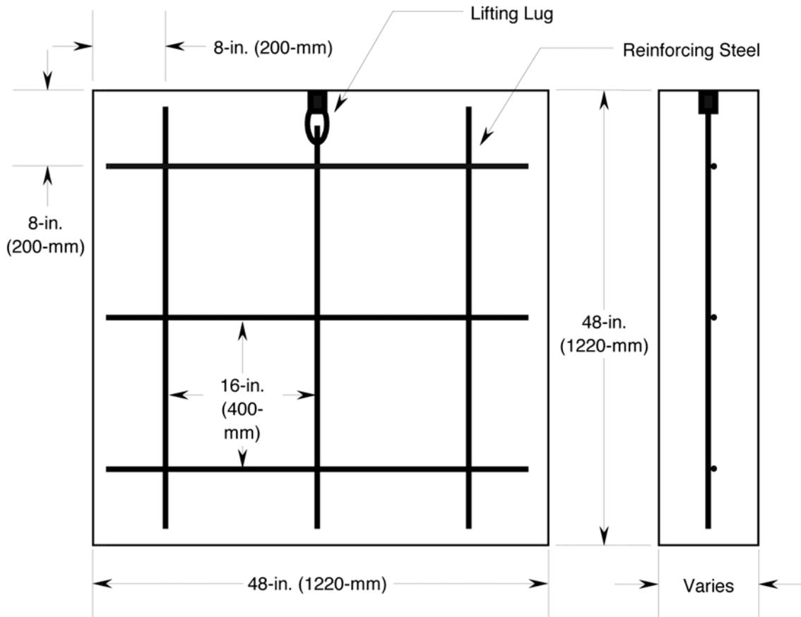
Figure 3. Layout of reinforcing steel in the ICF walls.
