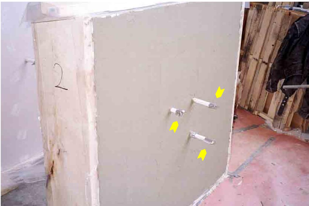
**Figure 23. Temporary caps on relative humidity ports in Wall No. 2.**
