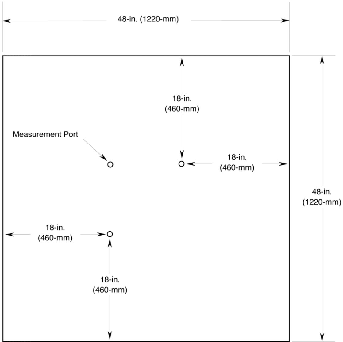
**Figure 6. Generalized layout of relative humidity ports in walls.**
