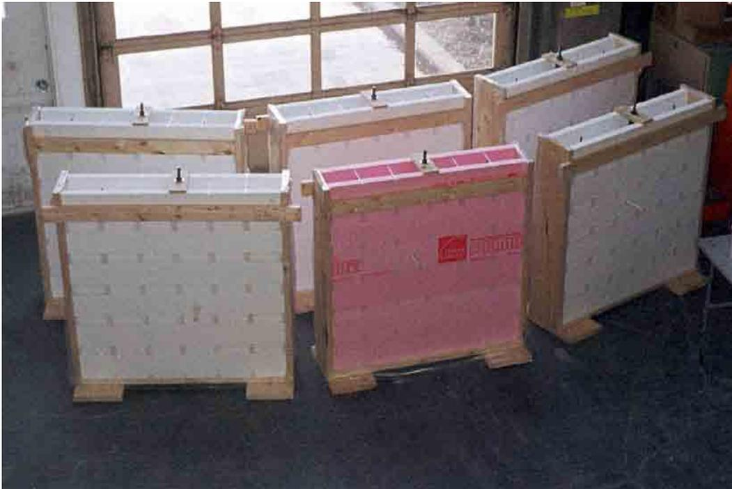
**Figure 5. ICF wall sections in wood forms with reinforcing steel installed.**
