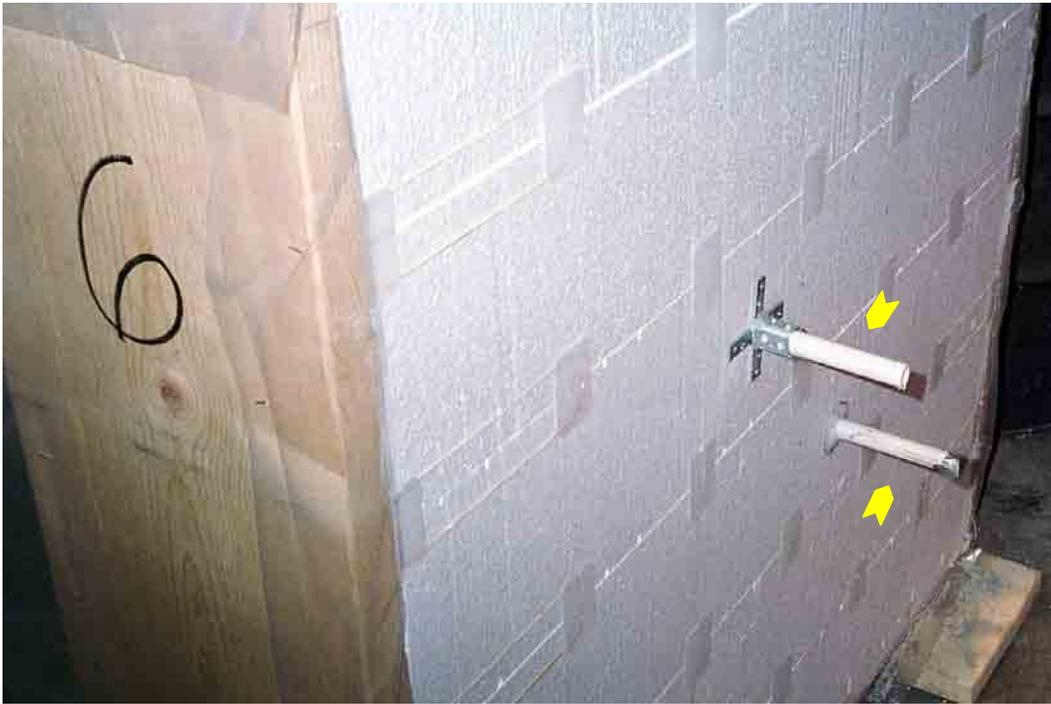
**Figure 7. Relative humidity ports installed in Wall No. 6.**
