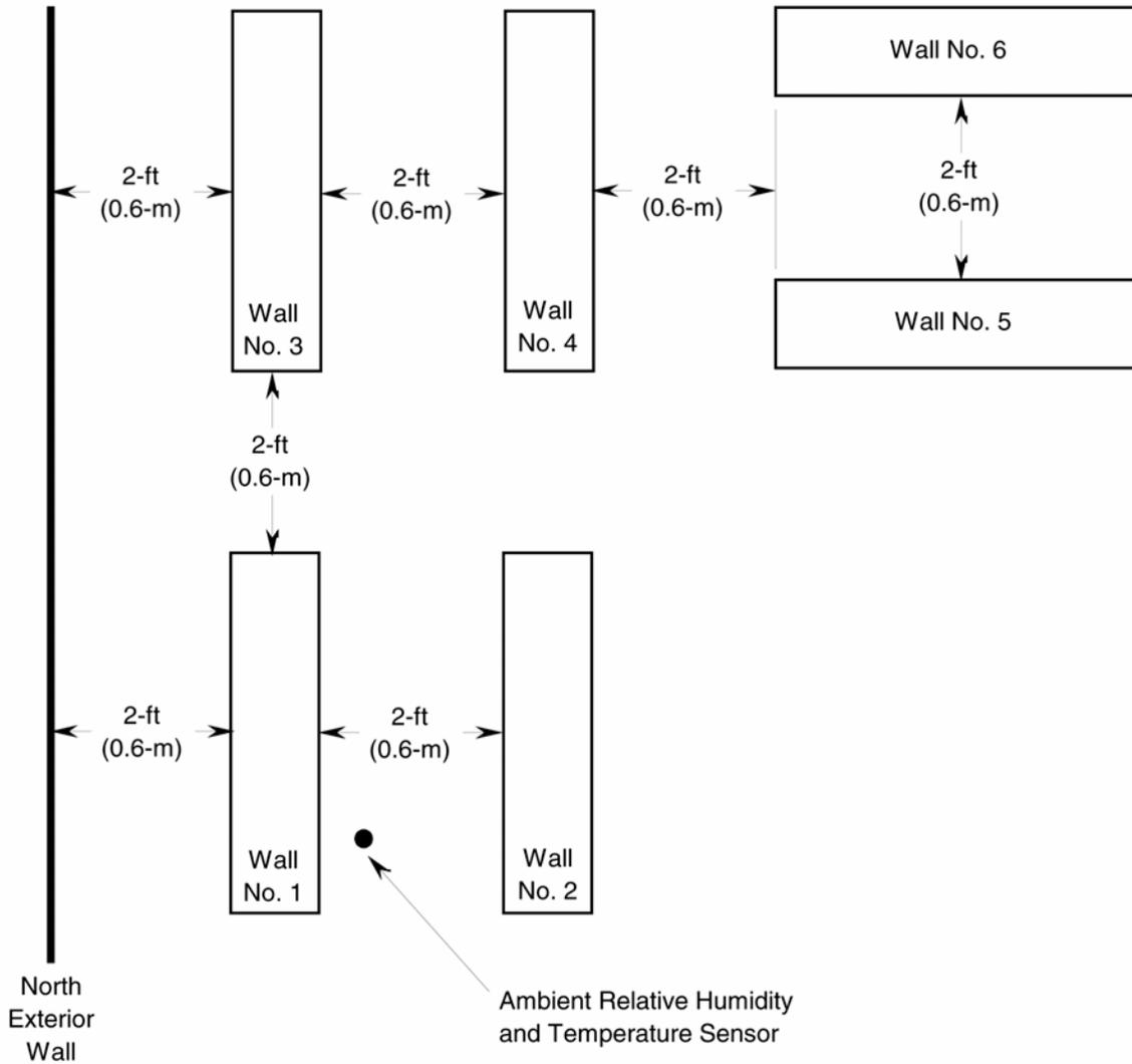
Figure 25. Layout of wall sections in storage environment.
