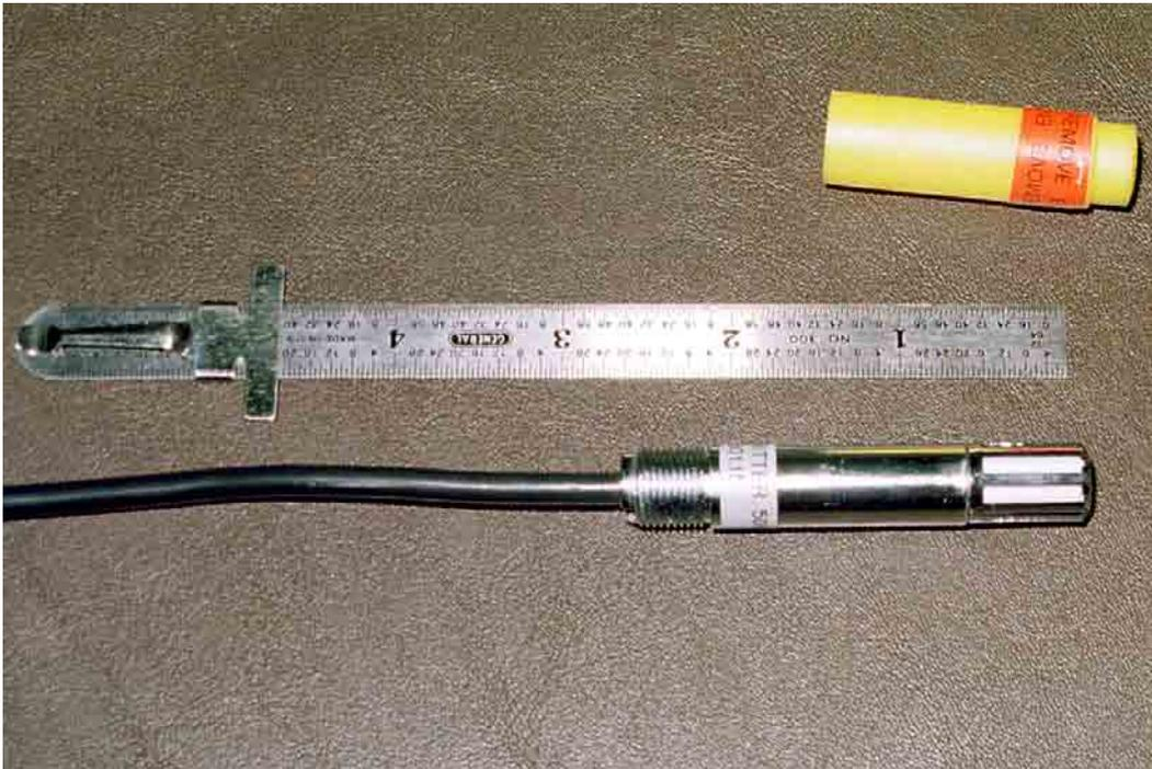
Figure 26. Relative humidity probe.
