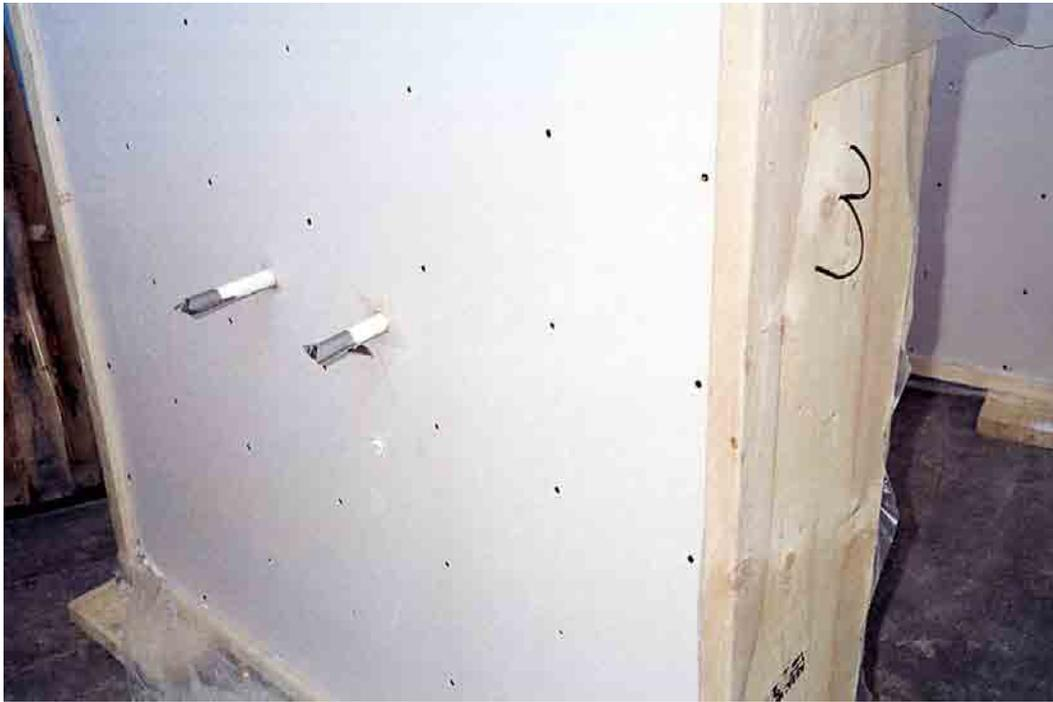
**Figure 14. Wall No. 4 with drywall installed prior to application of drywall compound.**
