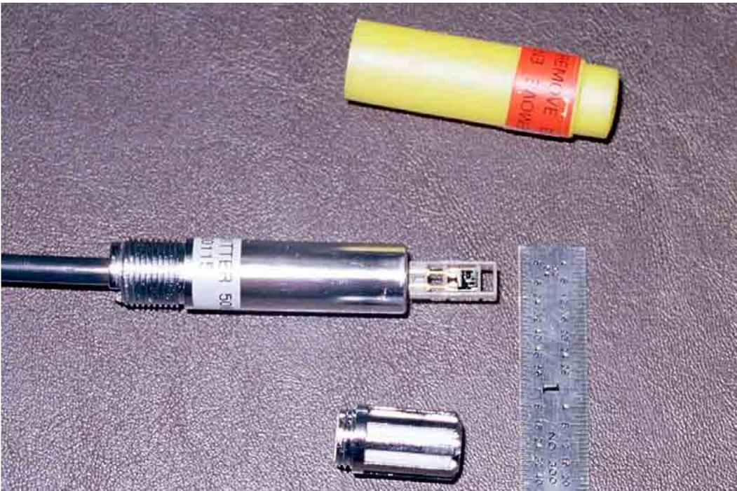
Figure 27. Relative humidity probe with the protective housing of the relative humidity sensor removed.
