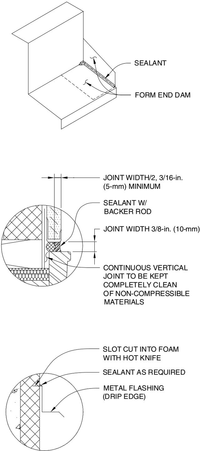
Figure D2. Typical head flashing end dam and sealant details.
