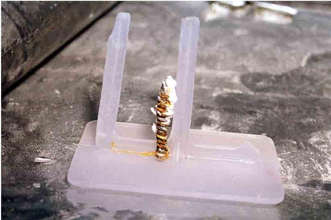
**Figure 28. Close-up of drywall screw showing corrosion.**
