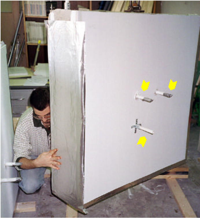
Figure 1. Photograph showing edge sealing being applied to a wall section with three measurement ports.
