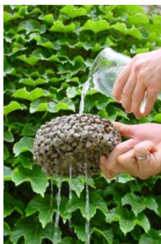
Figure 1 Pervious concrete used for heat island mitigation and stormwater management
