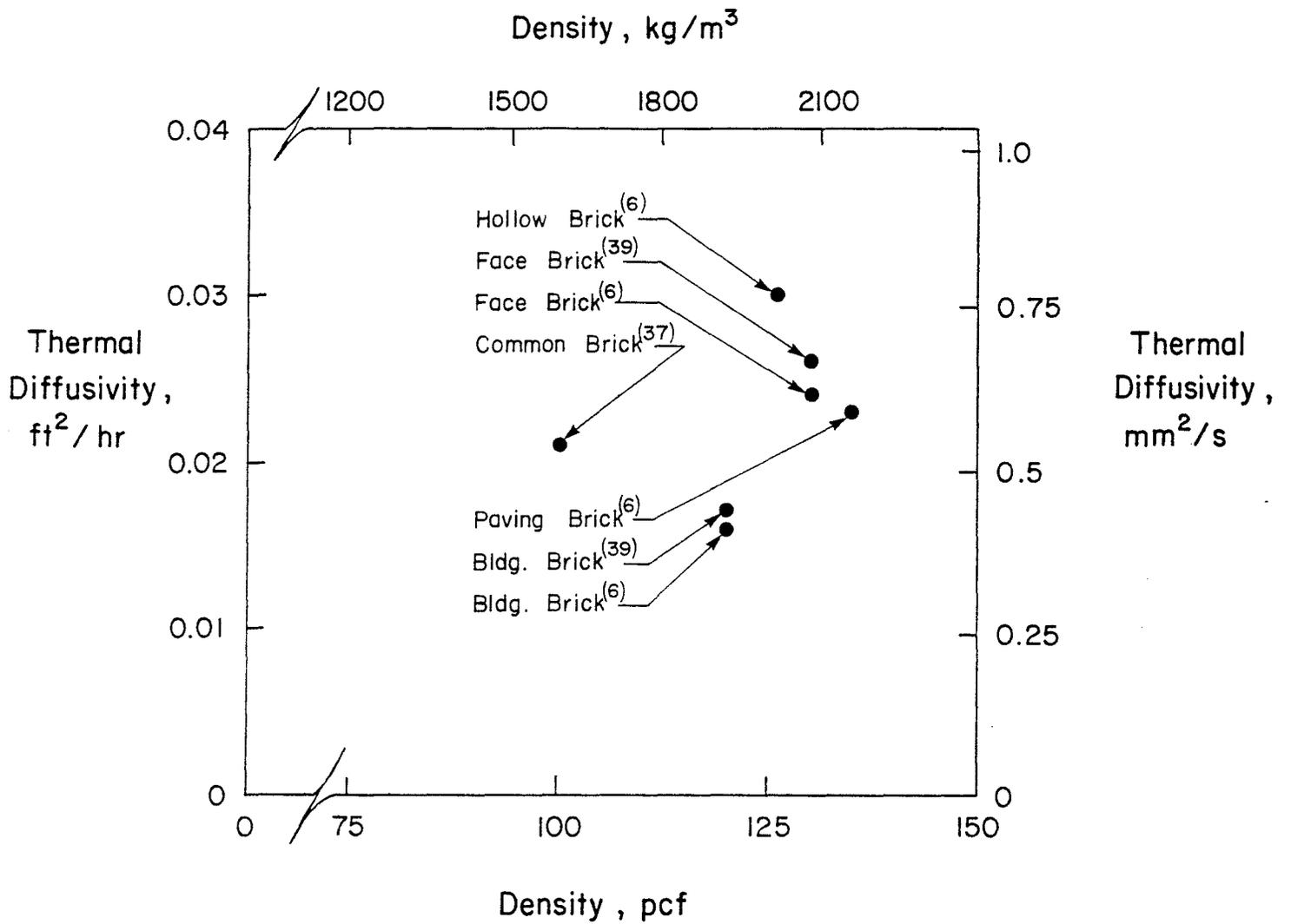
Fig. 25 Thermal Diffusivity of Clay Brick as a Function of Density
