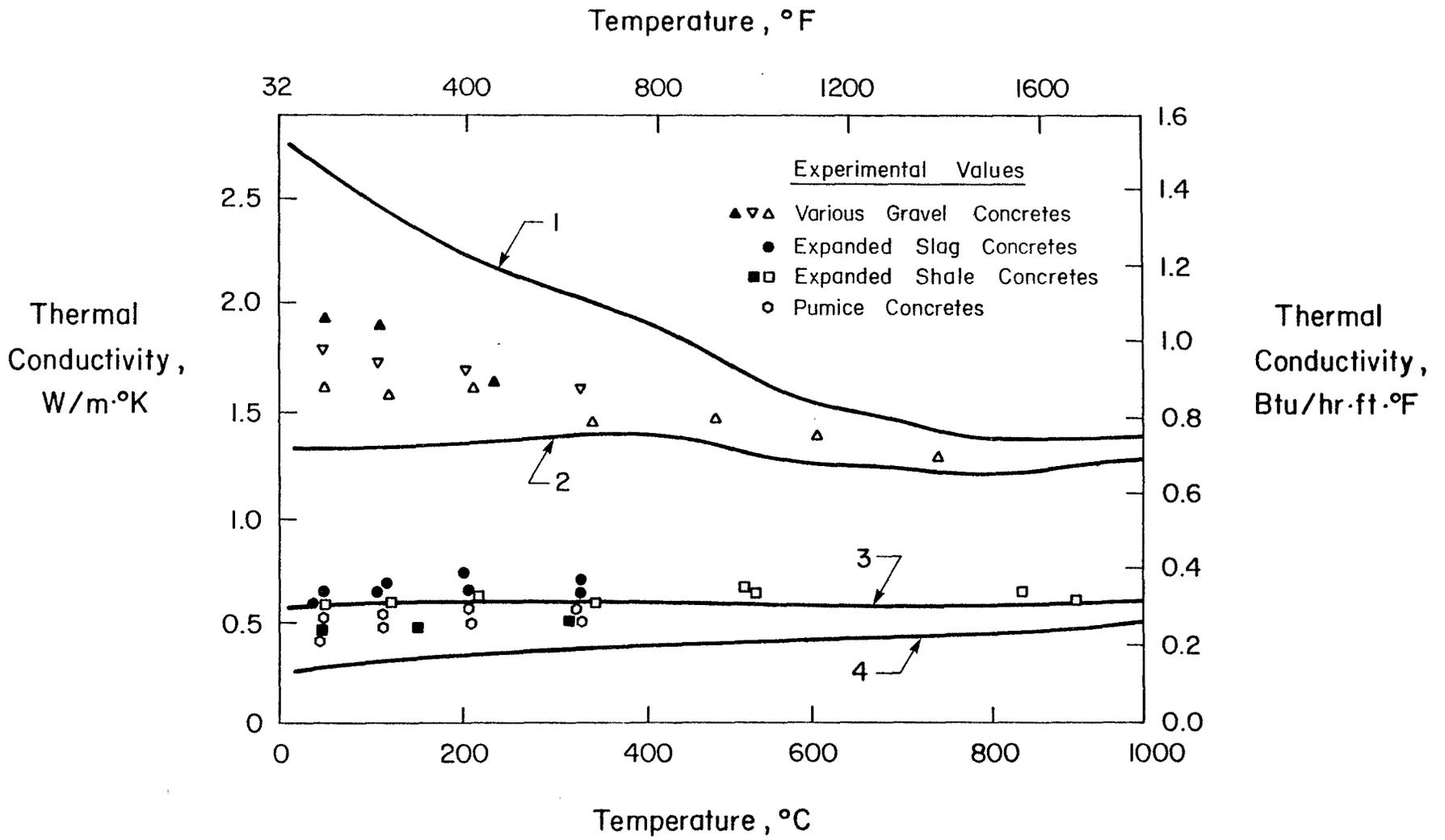
Fig. 24 Thermal Conductivity of Four "Limiting" Concretes as a Function of Temperature<sup>(35)</sup>
