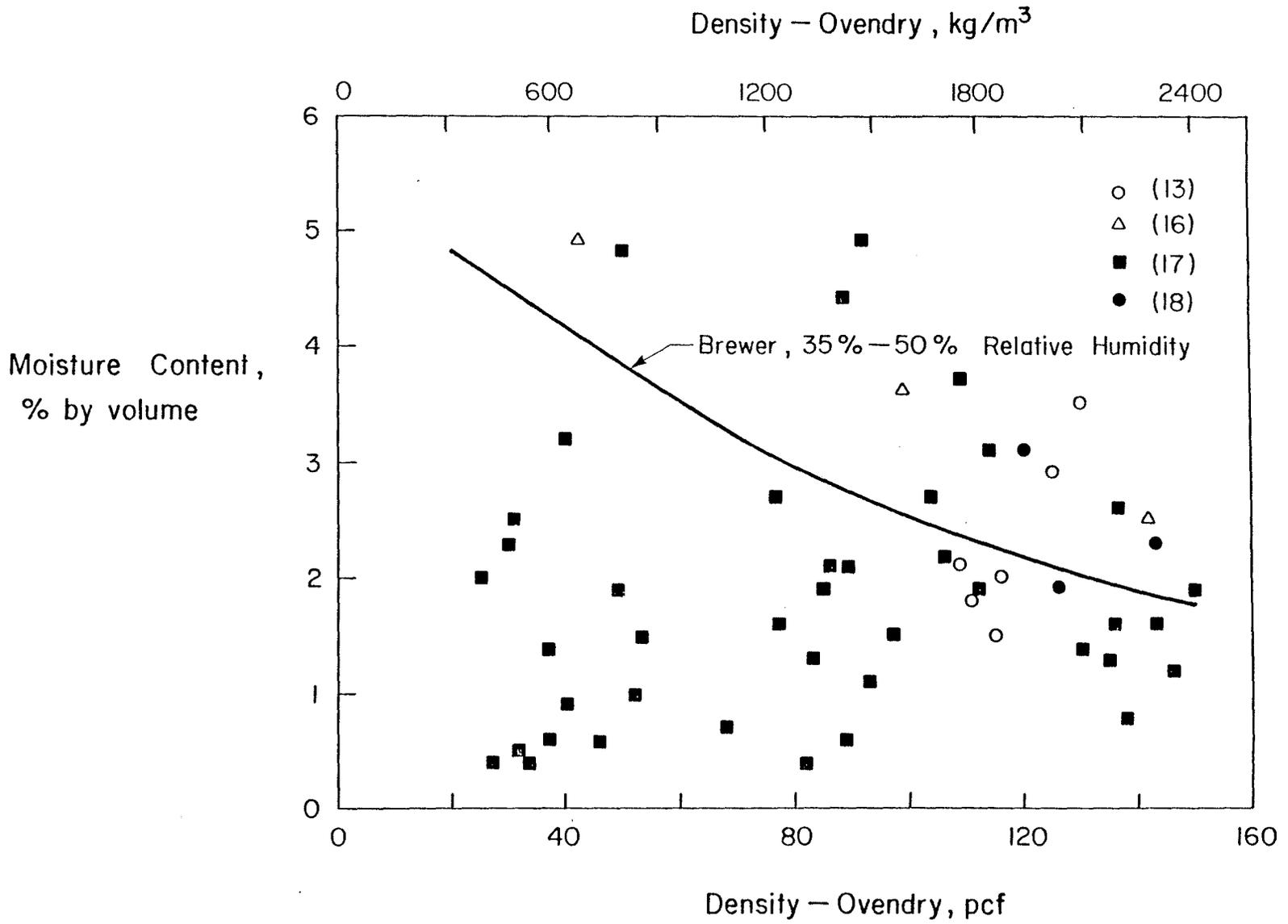
Fig. 8 Moisture Content of Normally Dry Concrete as a Function of Density
