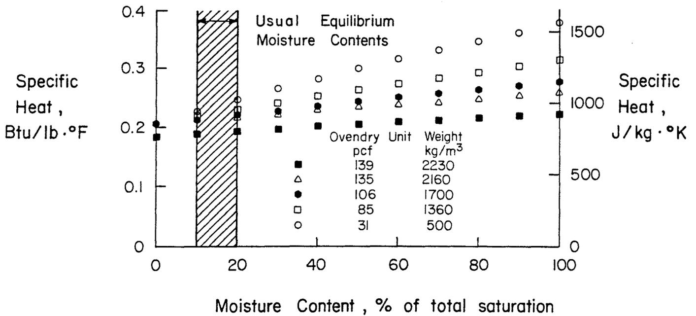
Fig. 6 Specific Heat of Concrete as a Function of Moisture Content<sup>(11)</sup>
