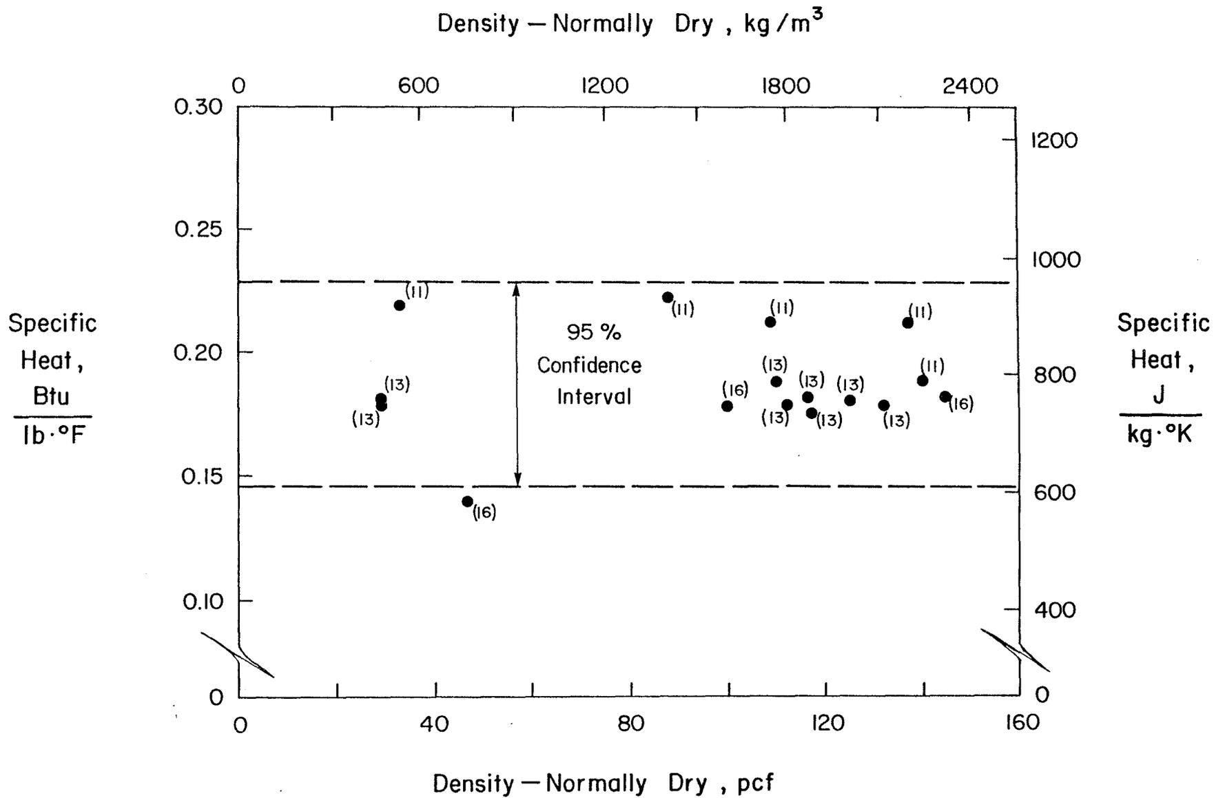
Fig. 10 Specific Heat of Normally Dry Concrete as a Function of Density - Using Moisture Contents of Normally Dry Concrete Proposed by Brewer
