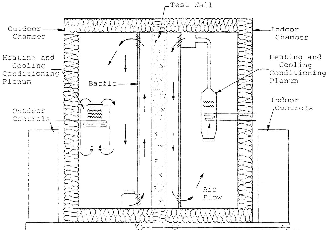
Fig. 16 Schematic Diagram of Calibrated Hot Box<sup>(26)</sup>
