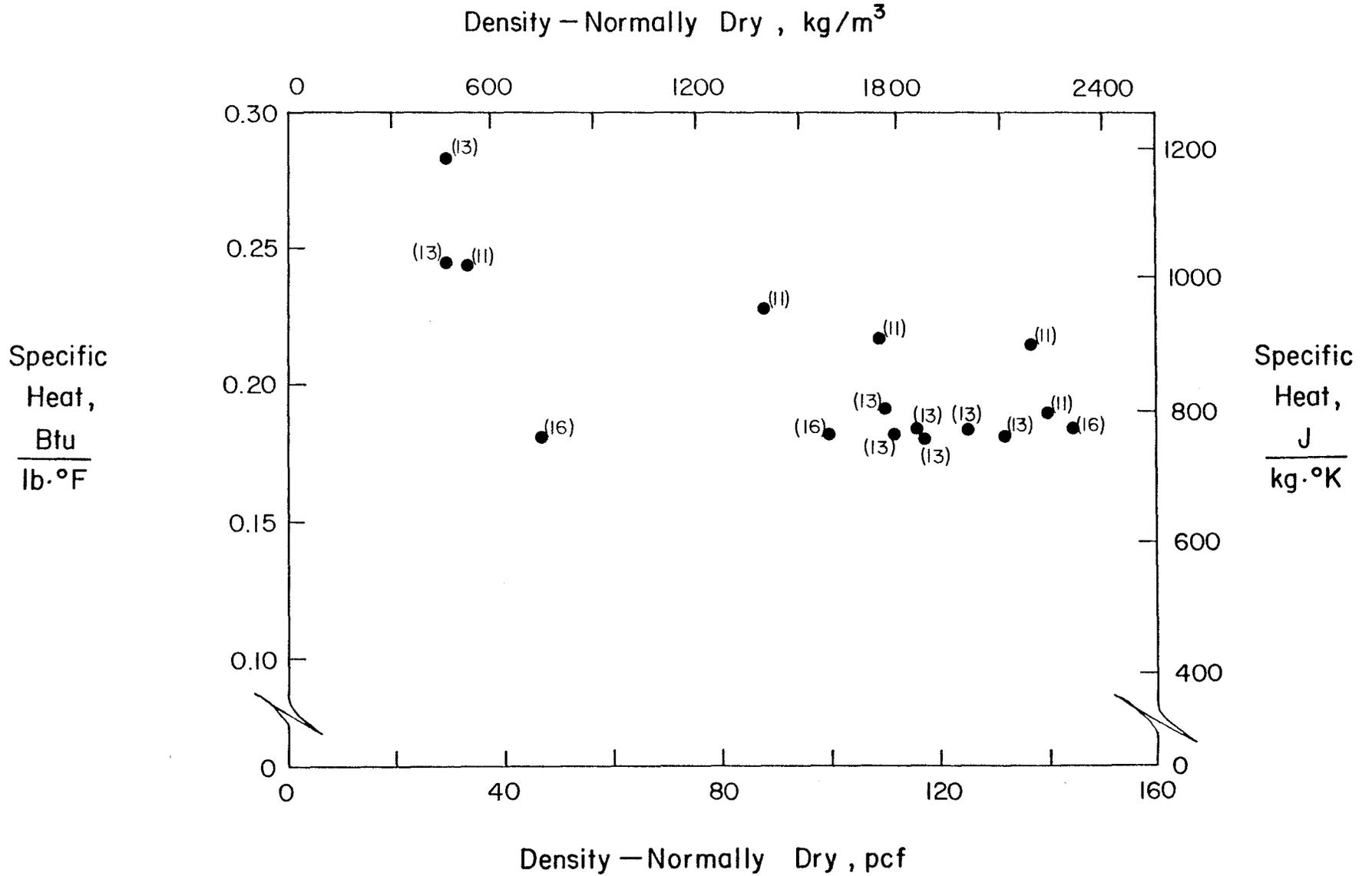
Fig. 11 Specific Heat of Normally Dry Concrete as a Function of Density - Moisture Content in Terms of Percent of Total Saturation is Constant
