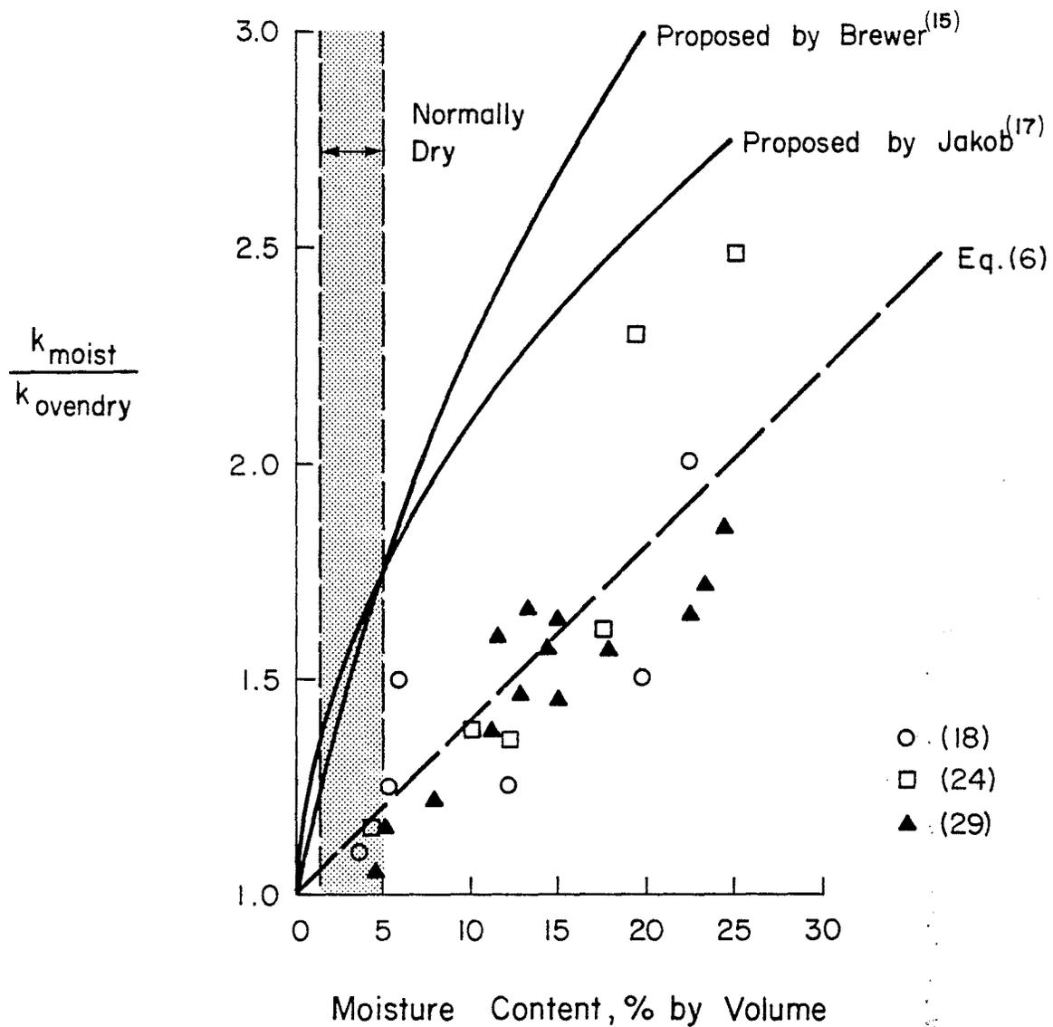
Fig. 21 The Ratio of the Conductivity of Moist Concrete to the Conductivity of Oven-dry Concrete as a Function of Moisture Content
