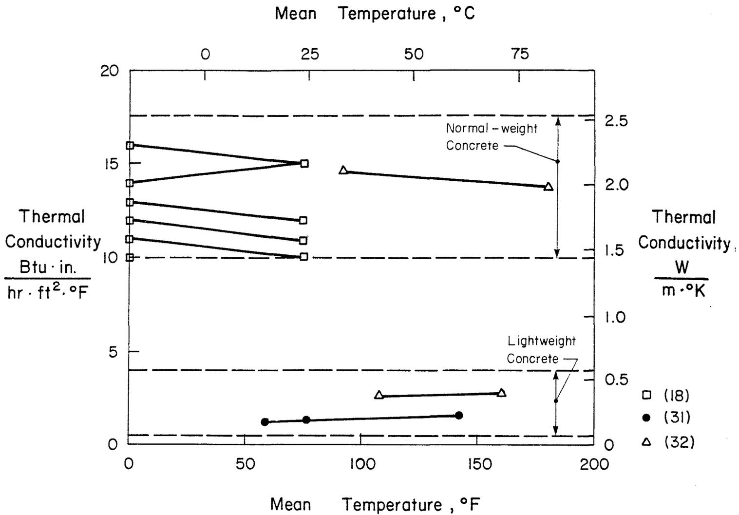
Fig. 23 Thermal Conductivity of Concrete as a Function of Temperature
