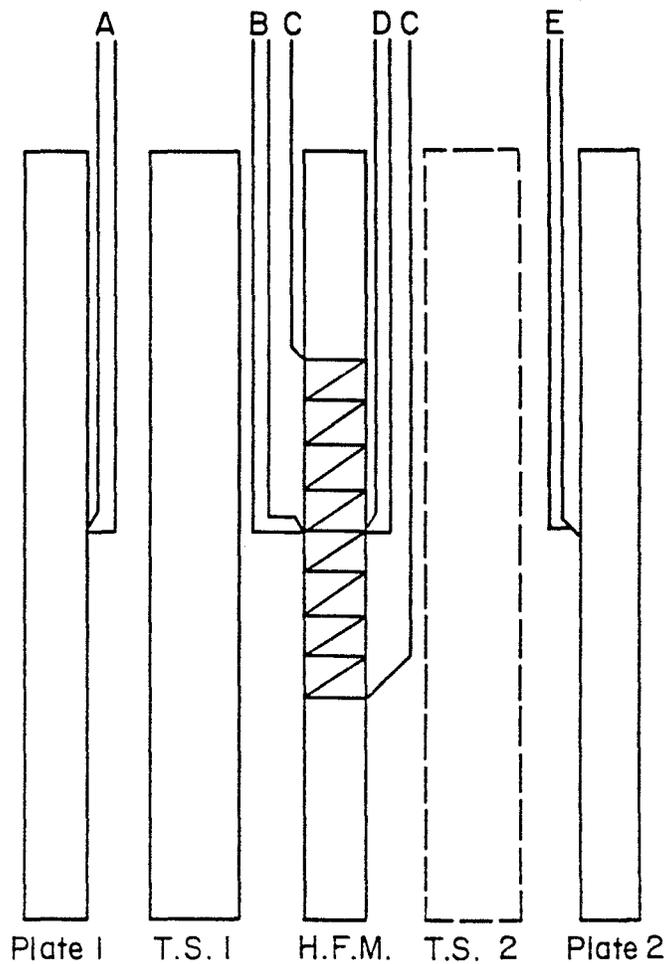
Plate 1-Controlled temperature plate at T1 (or T2)
