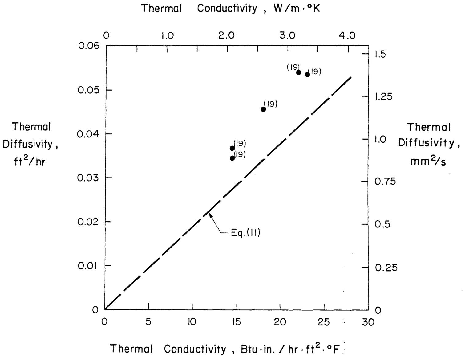
Fig. 27 Thermal Diffusivity of Concrete as a Function of Thermal Conductivity
