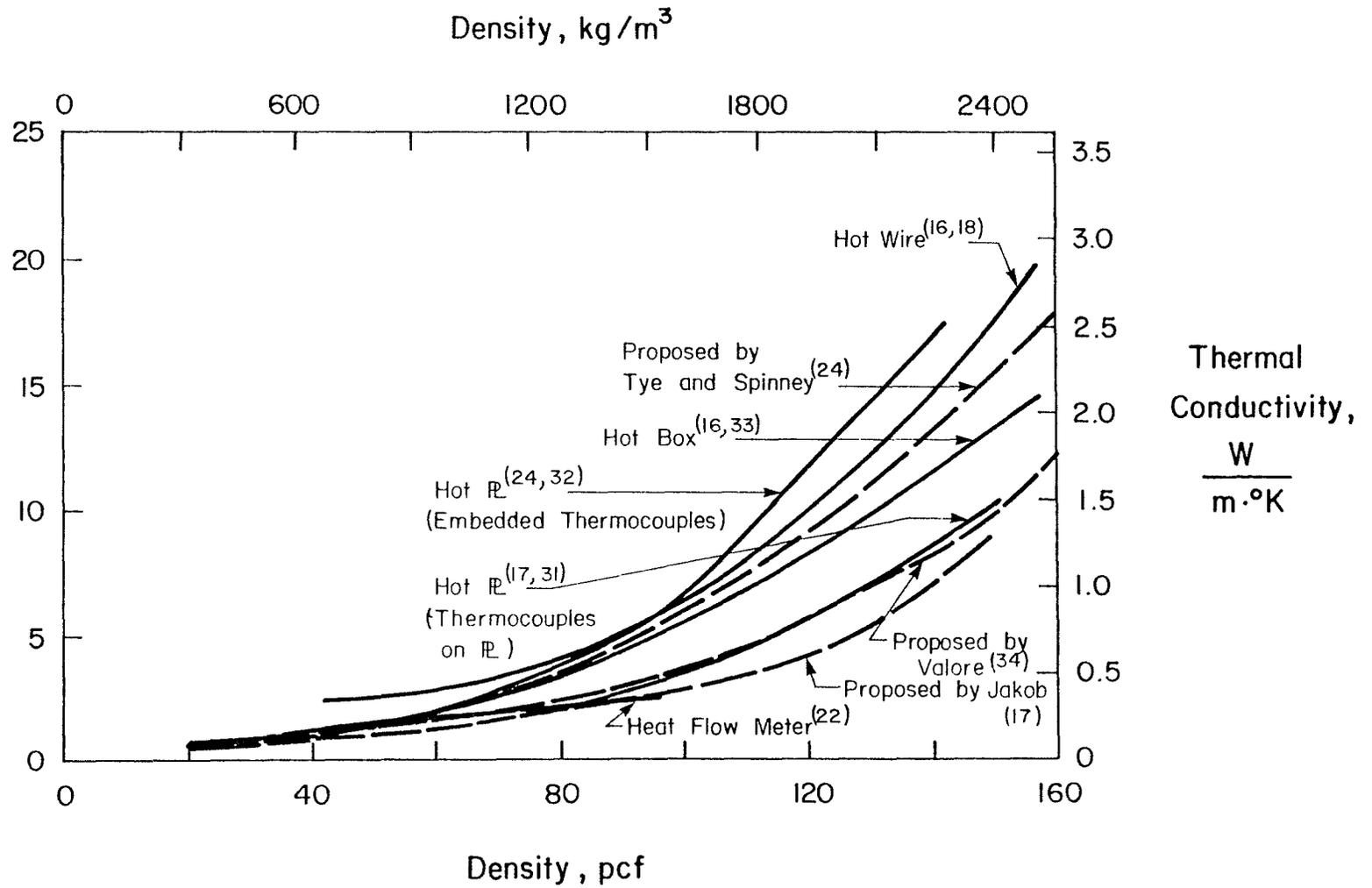
Fig. 22 Thermal Conductivity of Concrete as a Function of Density
