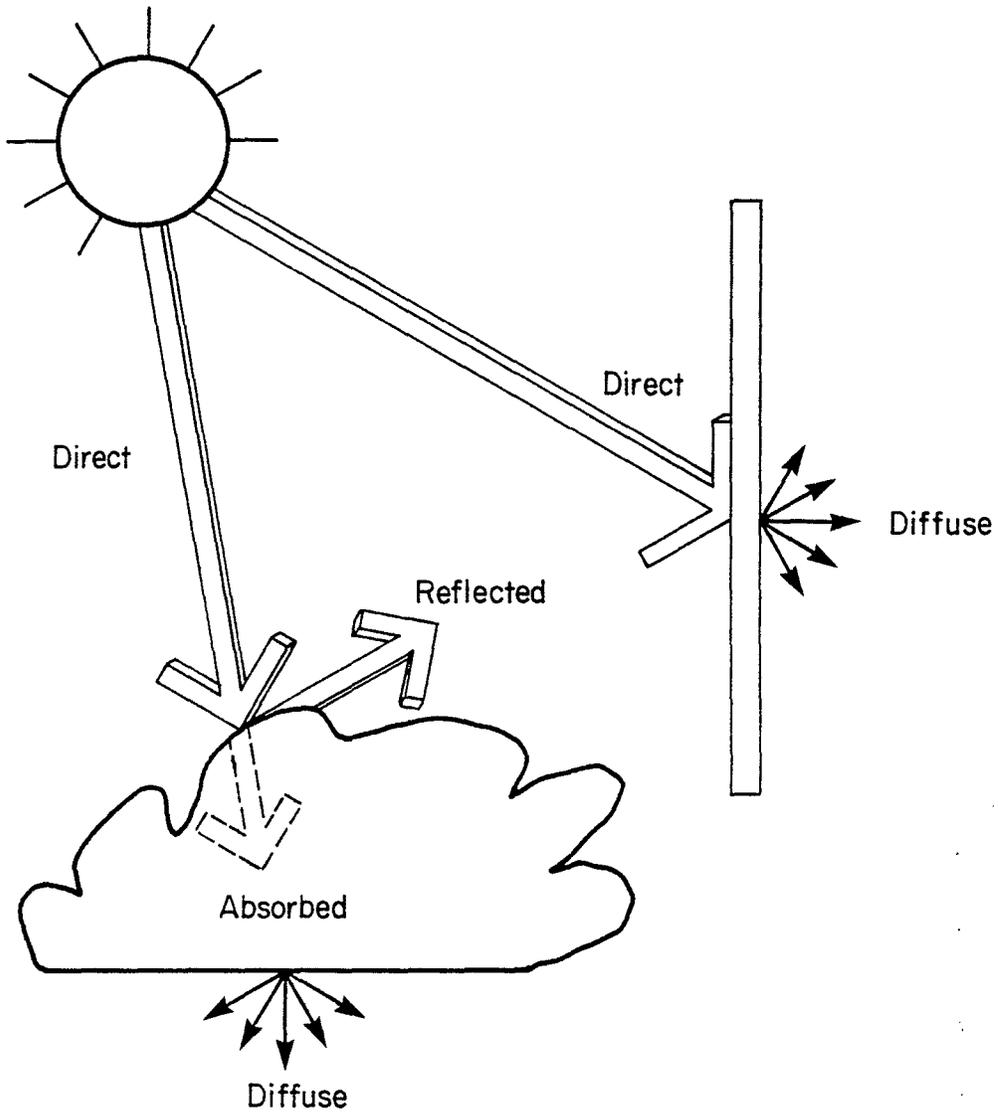
Fig. 3 Direct versus Diffuse Radiation
