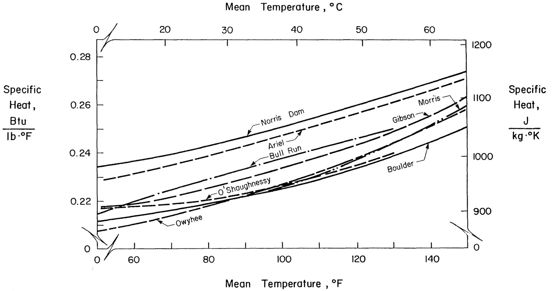
Fig. 13 Specific Heat of Concrete as a Function of Temperature (19)
