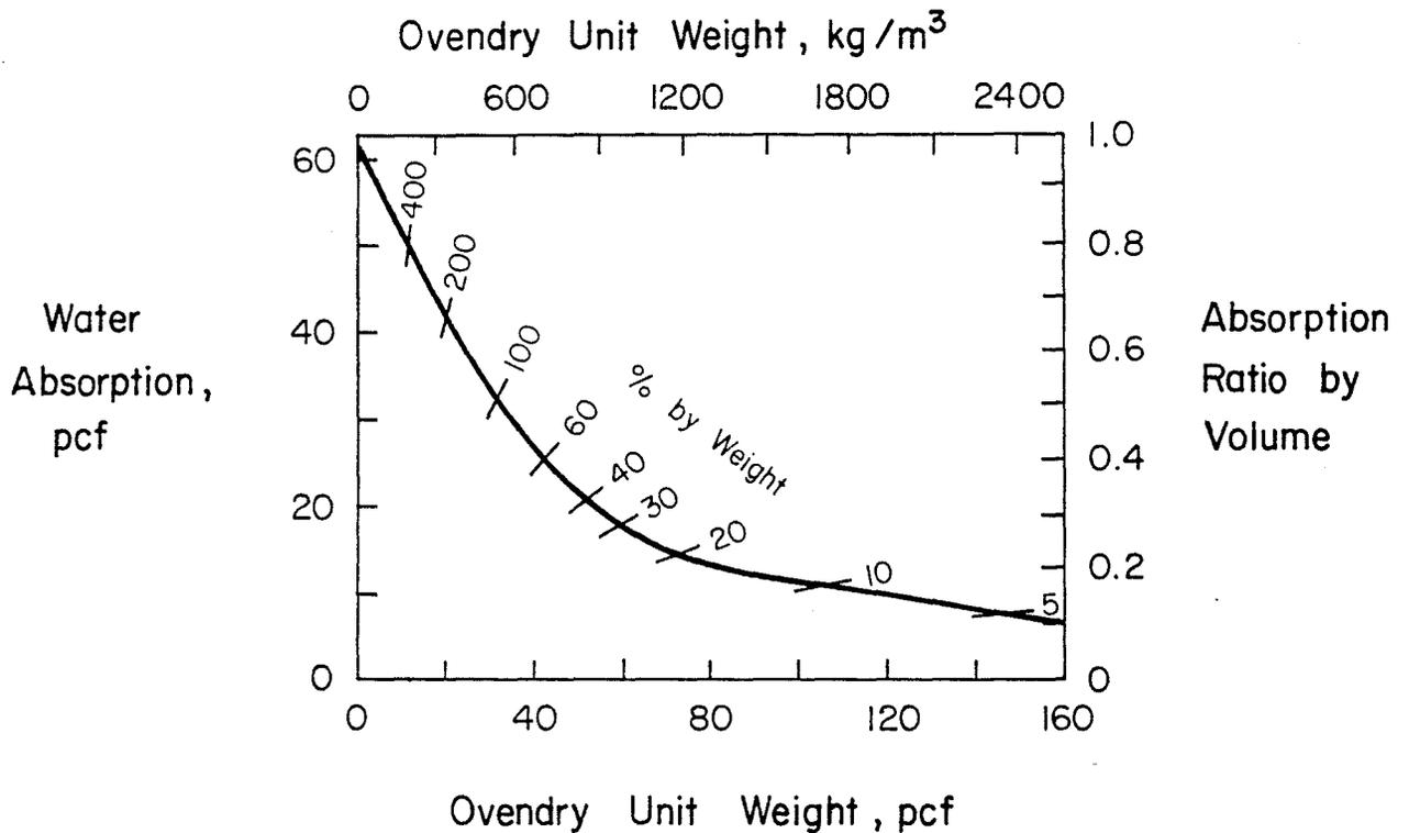
Fig. 7 Average Absorptions of Concretes<sup>(15)</sup>
