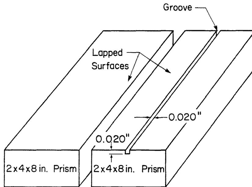
Fig. 18 Split Specimen Used in Hot Wire Method<sup>(28)</sup>
