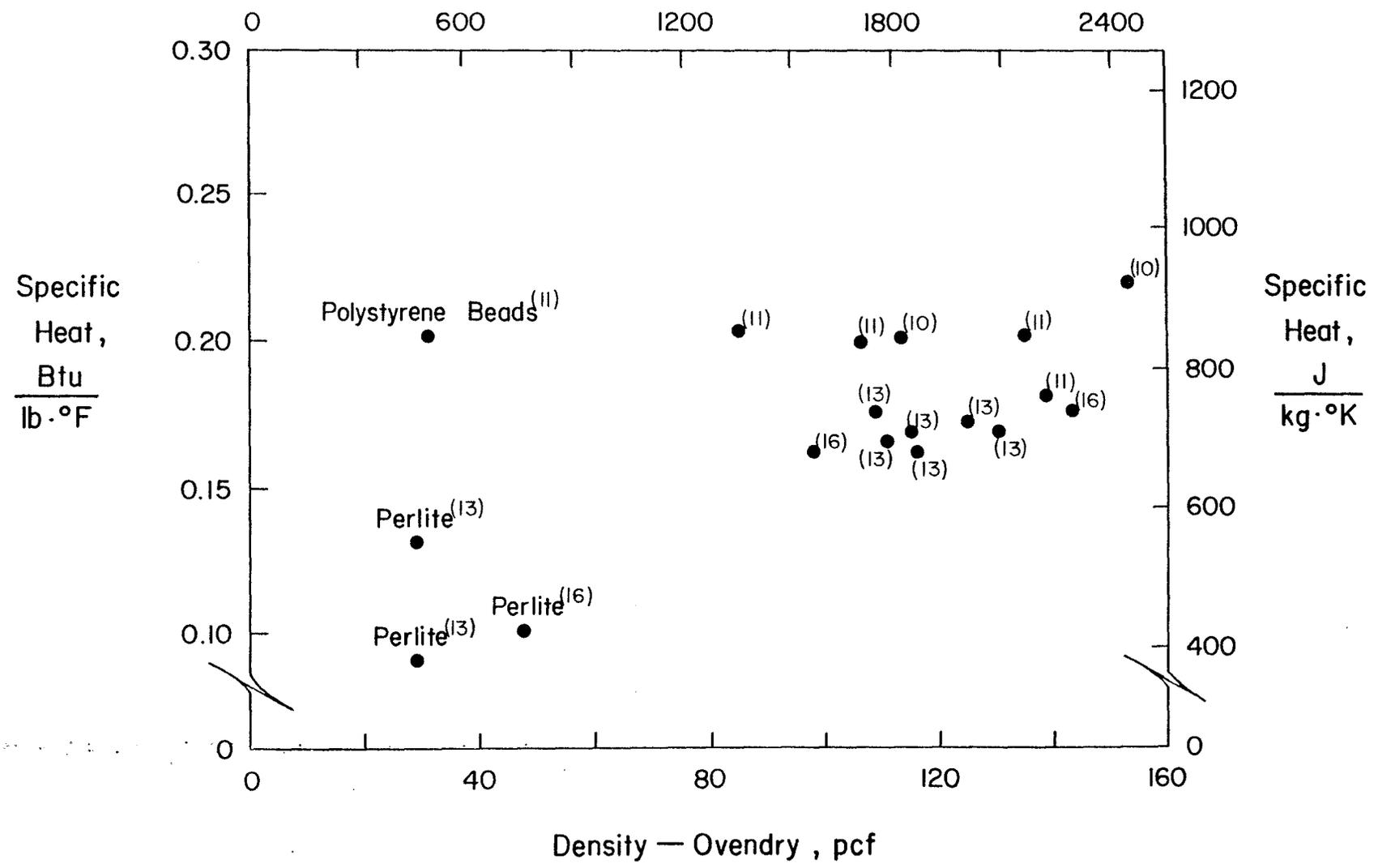
Fig. 9 Specific Heat of Ovendry Concrete as a Function of Density
