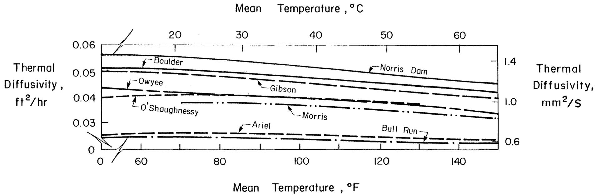
Fig. 28. Thermal Diffusivity of Concrete as a Function of Temperature (19)
