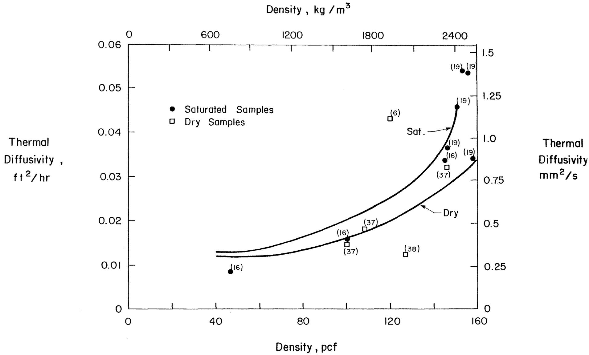
Fig. 26 Thermal Diffusivity of Concrete as a Function of Density
