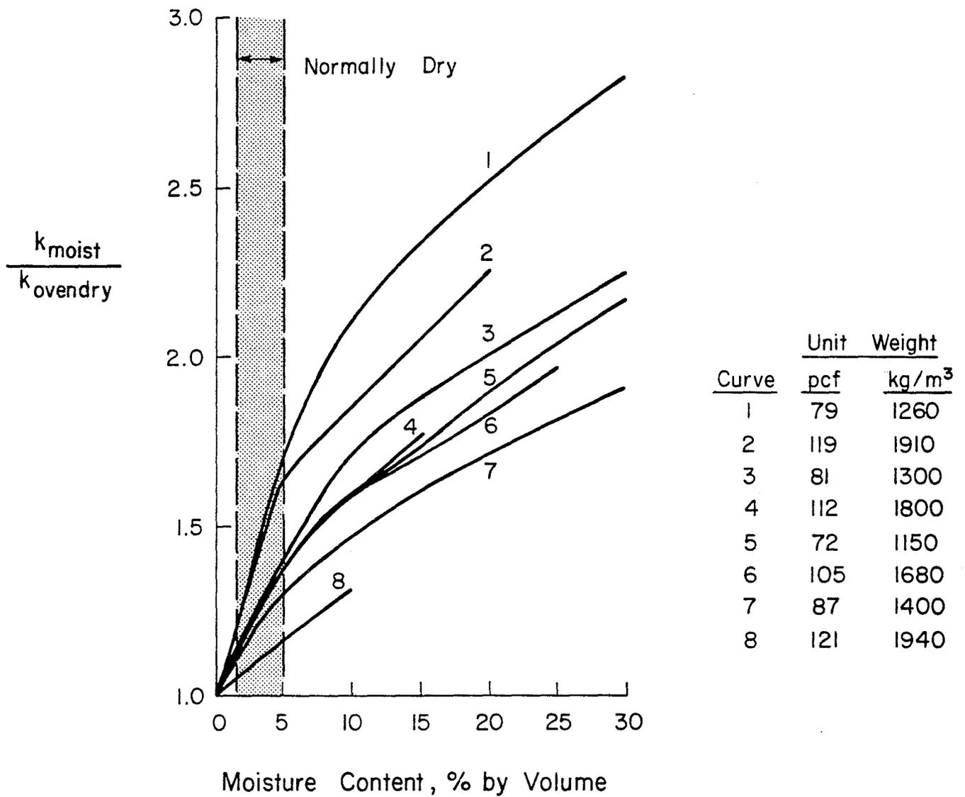
Fig. 20 The Ratio of the Conductivity of Moist Clay Brick to the Conductivity of Oven-dry Brick as a Function of Moisture Content(27)
