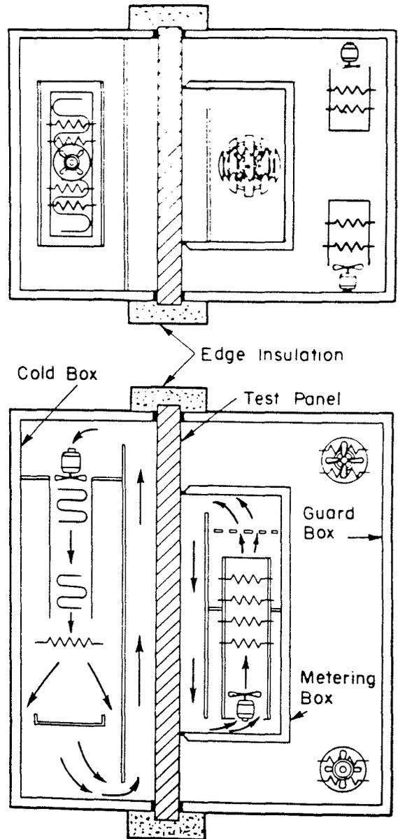
Fig. 15 Schematic Diagram of Guarded Hot Box (22)
