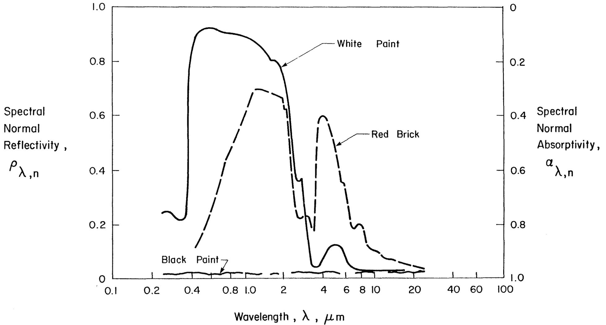
Fig. 34 Spectral Dependence of the Spectral, Normal Absorptivity and Reflectivity of White Paint, Black Paint, and Red Brick adapted from Incropera and DeWitt<sup>(4)</sup>
