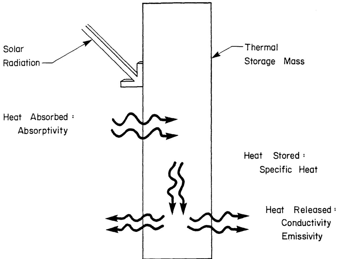
Fig. 2 Thermal Properties Relevant to the Thermal Storage Mass
