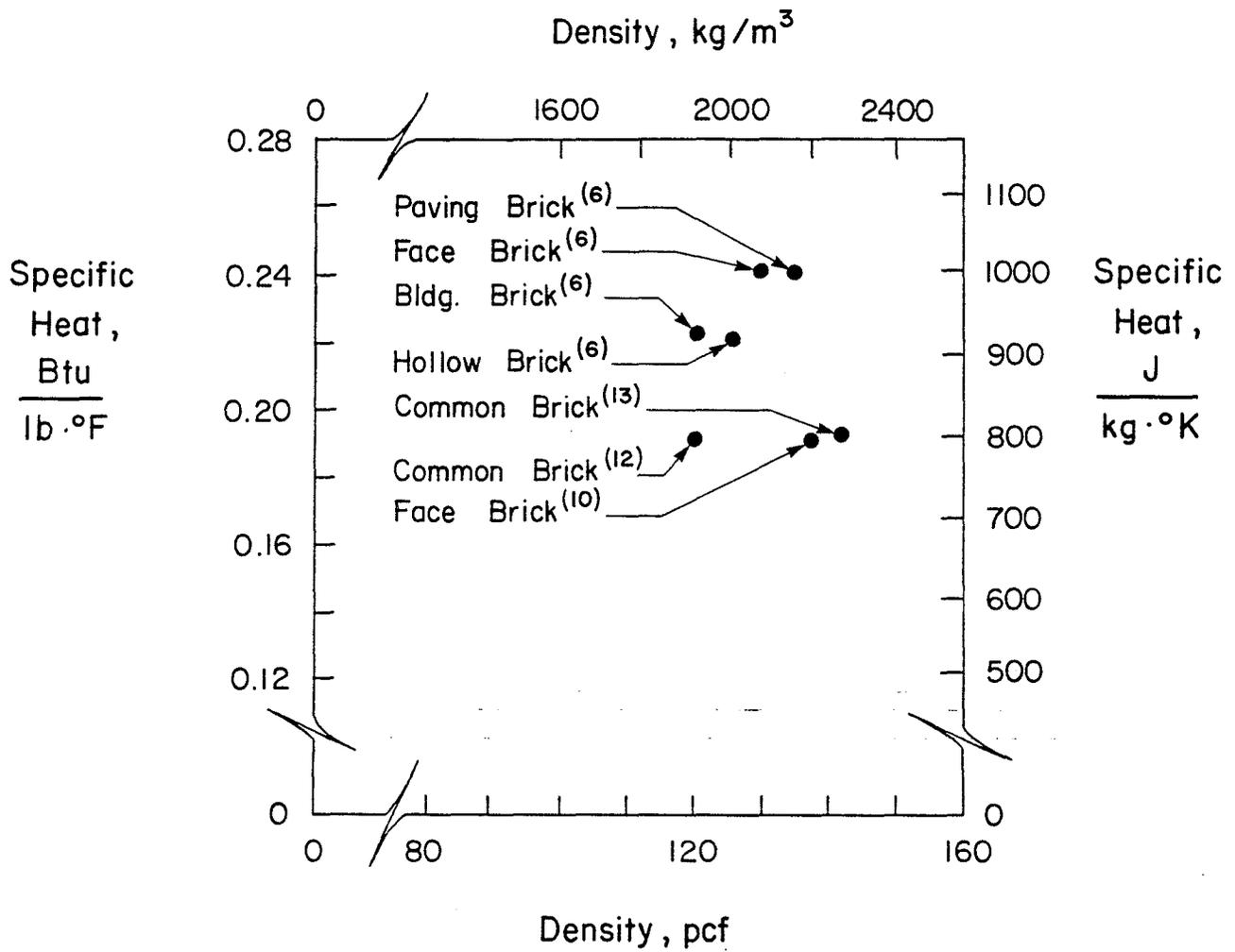
Fig. 5 Specific Heat of Clay Brick as a Function of Density
