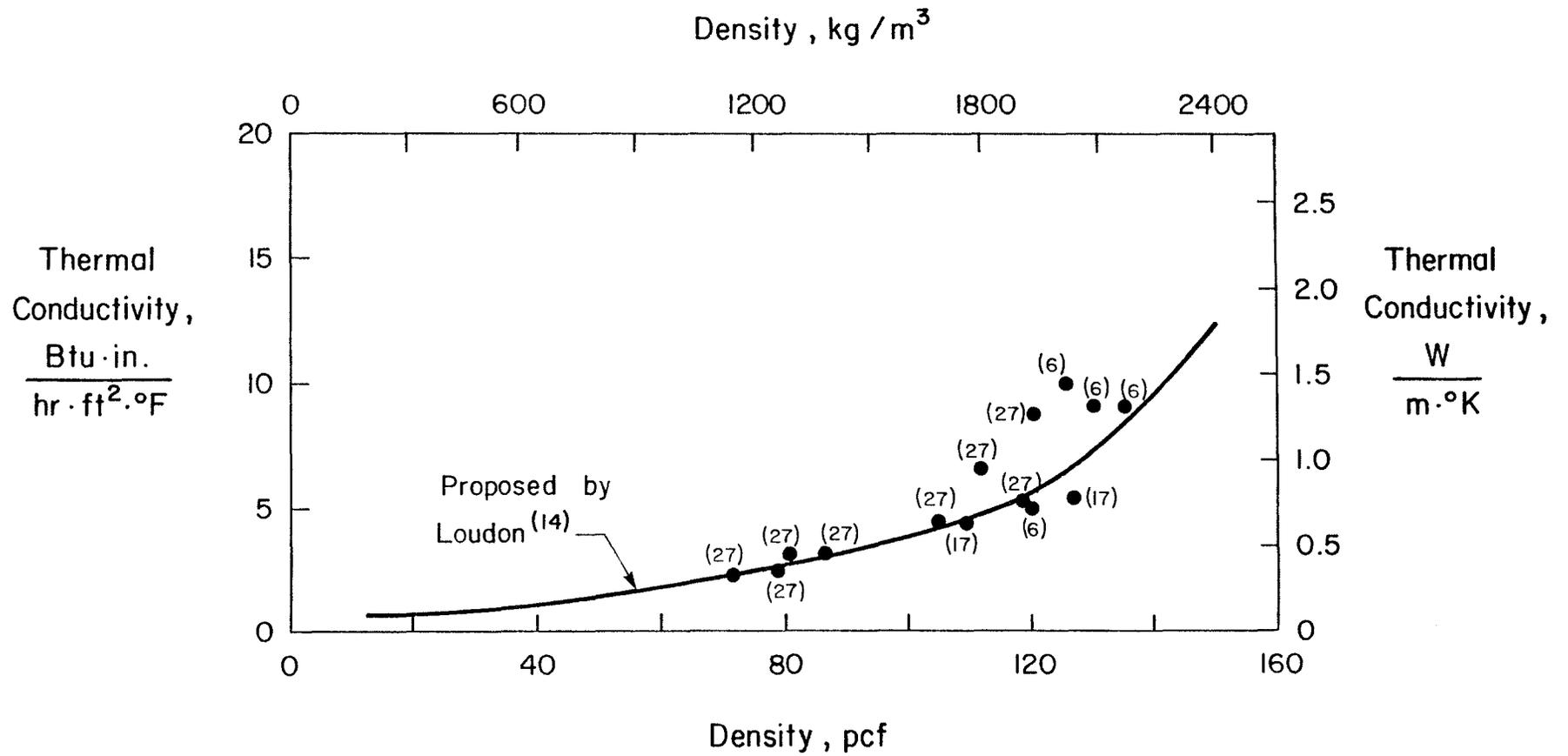
Fig. 19 Thermal Conductivity of Clay Brick as a Function of Density
